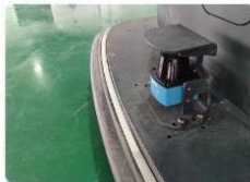
雷达系统 | Radar system 全向雷达，采用自然导航，无需调整基础设施，具备超高环境适应能力。 Omnidirectional radar, using natural navigation, no need to adjust infrastructure, with high environmental adaptability.
